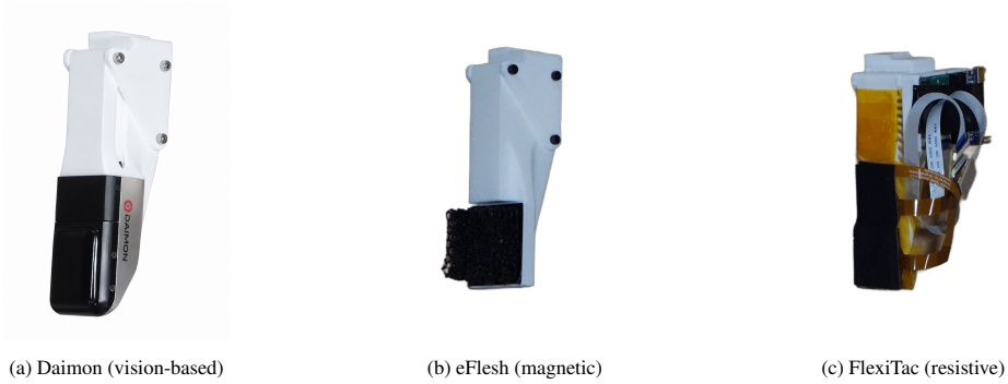
Figure 7: The three tactile sensors used in TACTX, each spanning a different transduction modality. All three are visually matched (black TPU/tape/elastomer) to remove cosmetic shortcuts and have roughly commensurate active sensing areas.
